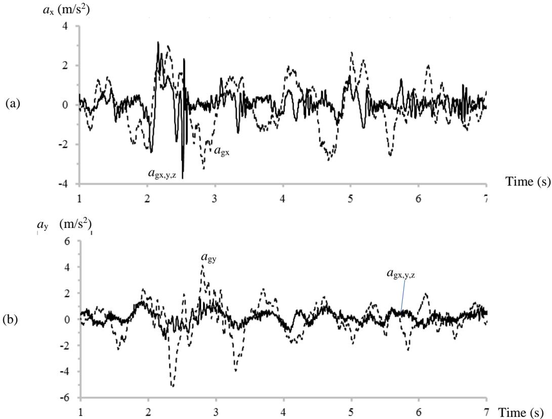
Figure 6. Influence of simultaneous three-directional ground excitation on the top acceleration of NSC in (a) the x- and (b) y-direction.
