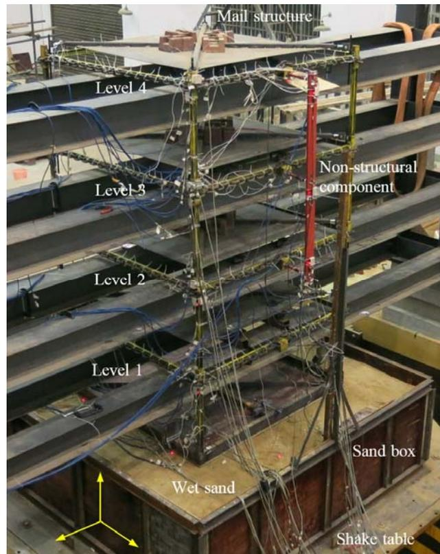
Figure 2. Main structure, non-structural component and sand box on shake table.
