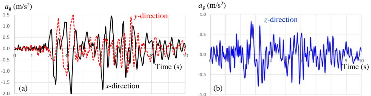
Figure 4. Ground excitation. (a) Horizontal components and (b) vertical component.
