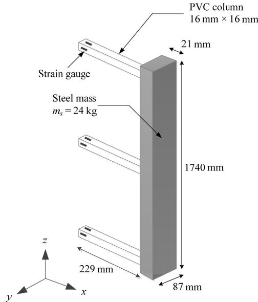
Figure 3. Sketch of the non-structural component.
