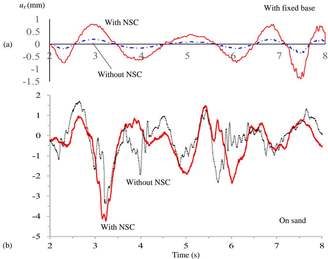
Figure 7. Influence of NSC and supporting soil on the vertical displacement at the NSC-main structure connection due to the horizontal ground excitation in the x-direction. Main structure with (a) an assumed fixed base and (b) on sand.
