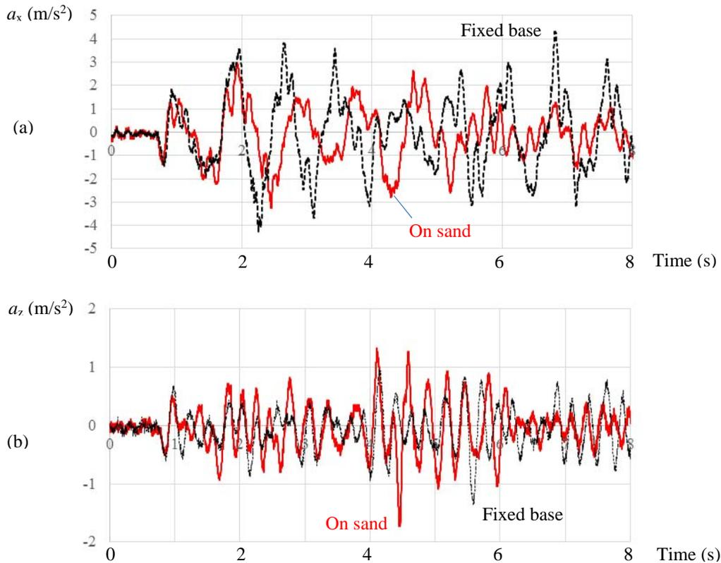
Figure 5. Influence of supporting soil on the top acceleration of the NSC (a) in the x-direction and (b) the vertical direction due to the horizontal ground excitation in the x-direction.
